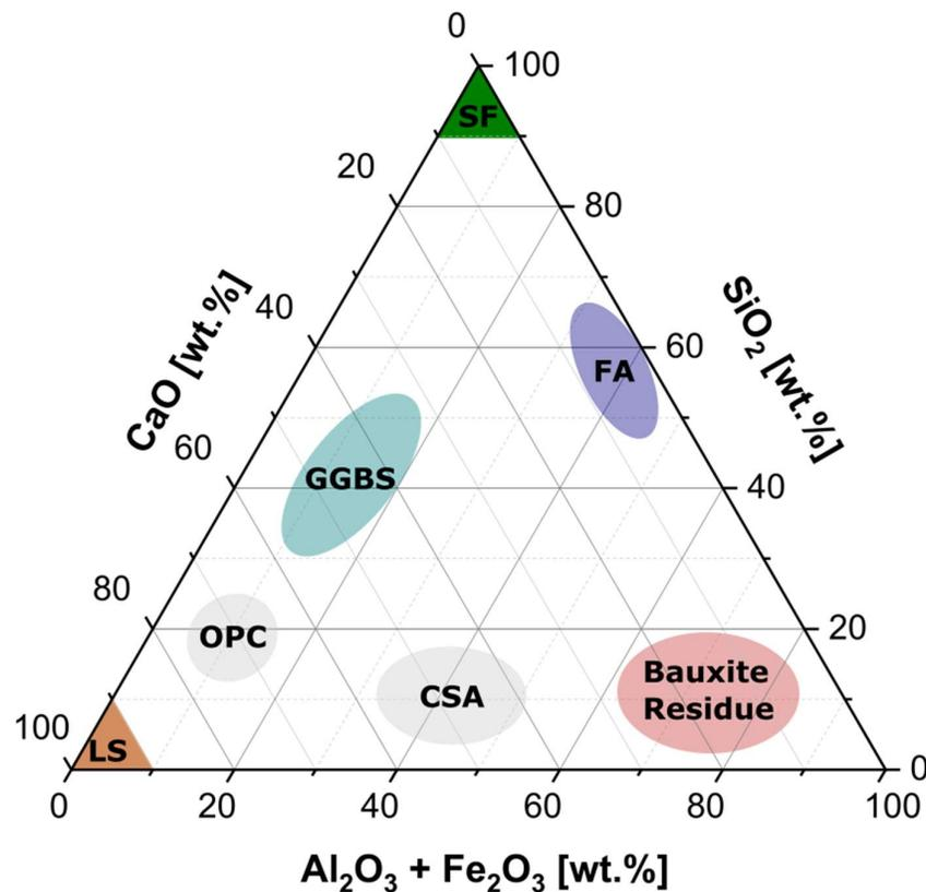
Figure 2 Ternary diagram of the most important oxides present in OPC systems. The difference of BR composition from traditional SCMs like BFS is illustrated schematically
