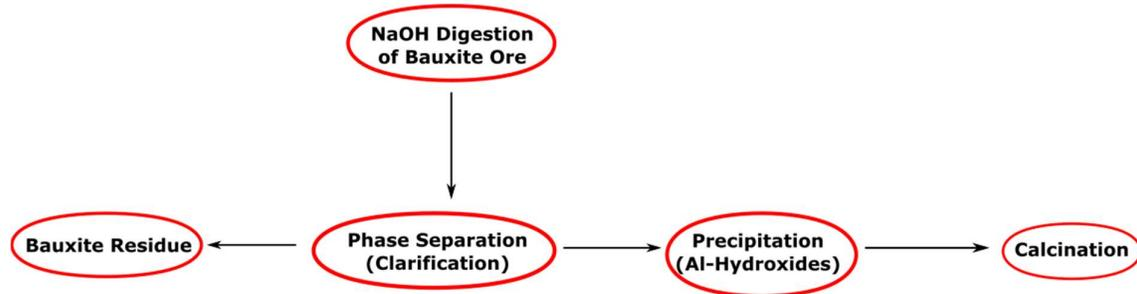
Figure 1 Scheme of the Bayer-Process leading to the production of alumina
